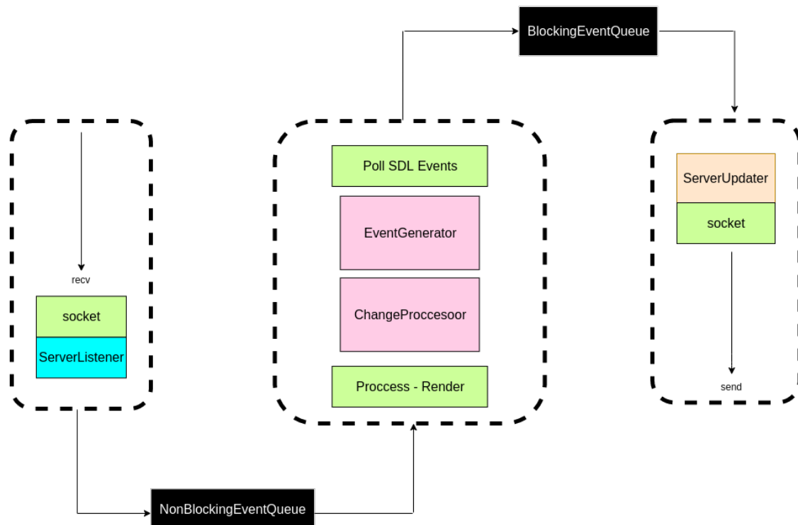
Diagrama general de threads del Cliente
